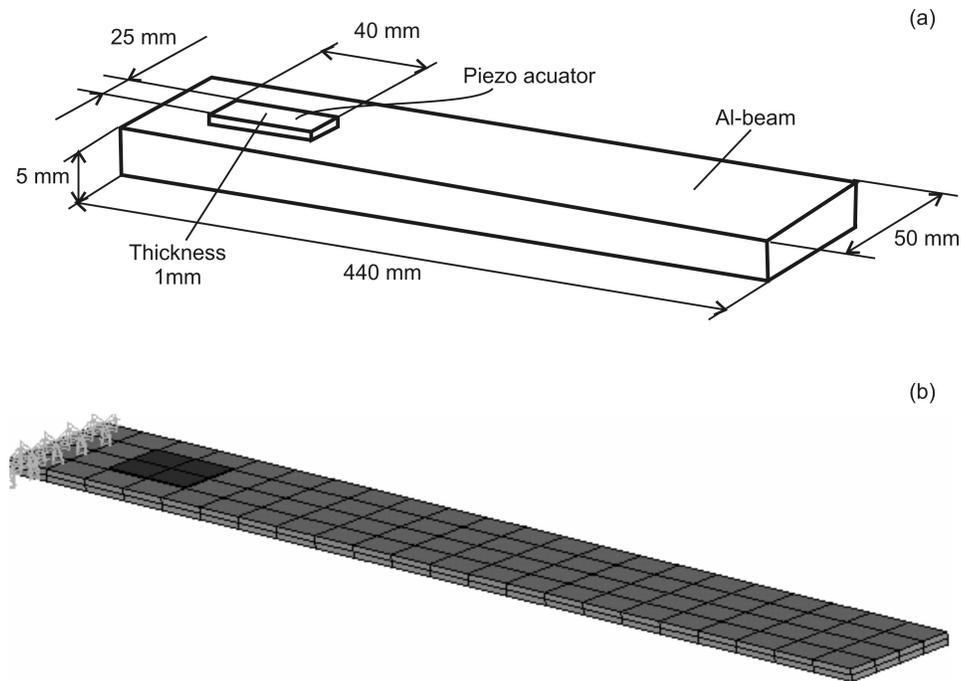
Fig. 6. Geometry of an aluminium beam with piezo actuator and finite element model: (a) geometry of the smart beam, (b) finite element model.
