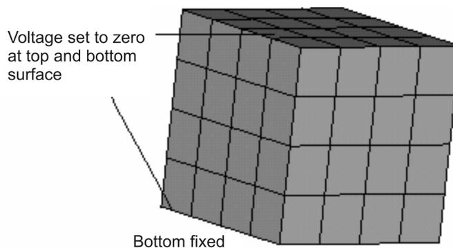
Fig. 5. FE model of piezoelectric transducer.
