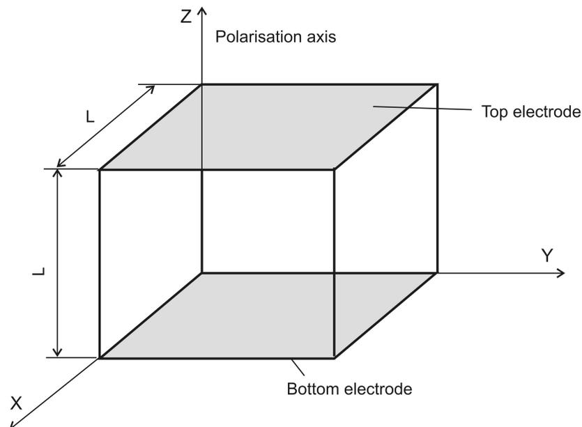
Fig. 4. Geometry of piezo transducer.
