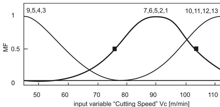
Fig. 3. MF – membership function (cutting speed).
